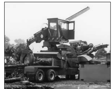
Wichita mechanical PTO handles shock and heavy loads for wood chippers.
