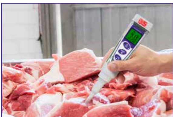
pH 5 FOOD - penetration electrode
