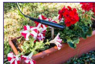
Soil conductivity with VPT Soil
