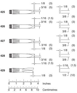
All dimensions are in inches. Bracketed dimensions are in millimetres.
