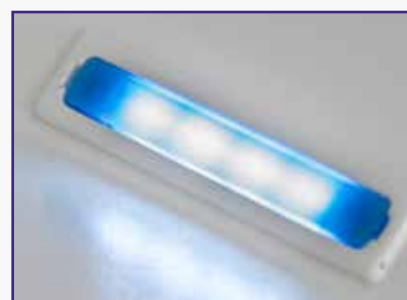
Visual signal of end of centrifugation
