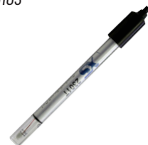
2301 T Conductivity cell, Temperature sensor integrated Cable 1 m Measuring range: 10µS...200 mS cod: 50004002
