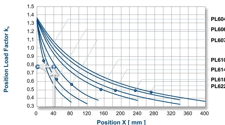
If the radial force F<sub>2r</sub> is not exerted on the center of the output shaft, then X is the distance measured from the output seal.
