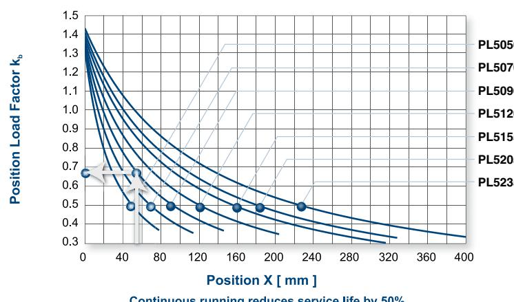
If the radial force  $F_{2r}$  is not exerted on the center of the output shaft, then  $X$  is the distance measured from the output seal.
