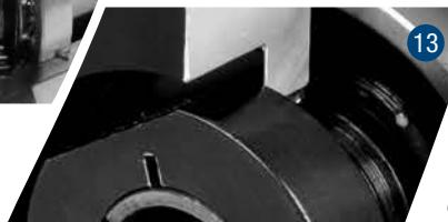
**Patented output sealing systems design** eliminates friction and heat generation which is accomplished by applying a hi-tech Titanium Carbon Nitride coating to all output contact surfaces. The TiCN coating reaches a hardness of 3000Hv and is ground to Ra 0.2µm finish to ensure sealing.
