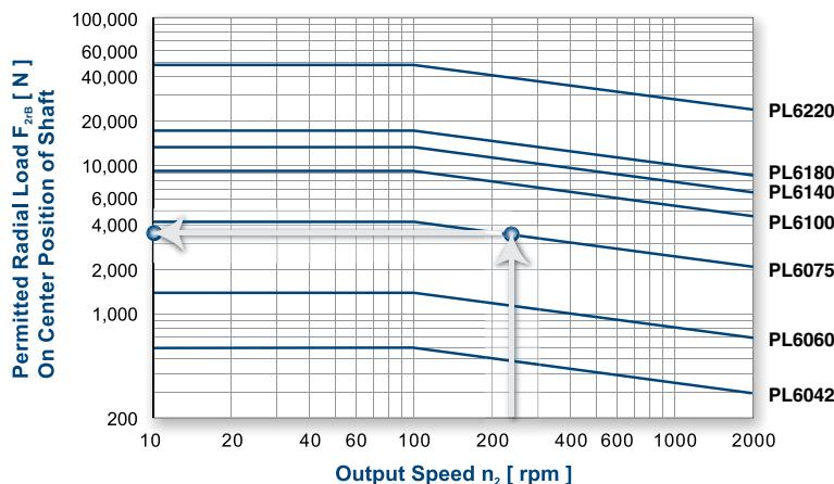
If the radial force F<sub>2r</sub> is exerted on the center of the output shaft, then X=0.5 x L.
