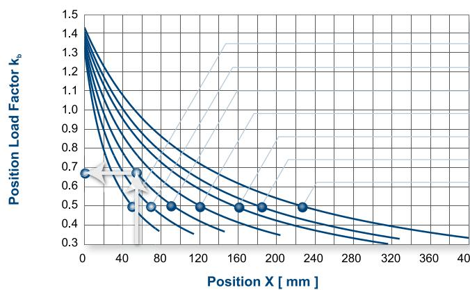
If the radial force  $F_{2r}$  is not exerted on the center of the output shaft then  $X$  is the distance measured from the output seal.
