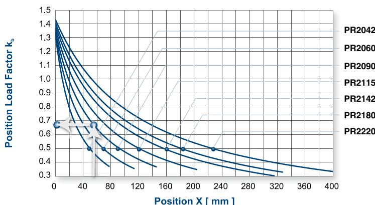
If the radial force  $F_{2r}$  is not exerted on the center of the output shaft, then  $X$  is the distance measured from the output seal.
