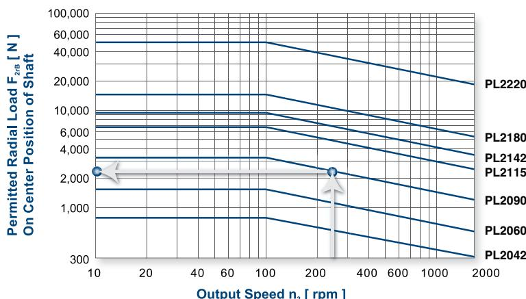
If the radial force  $F_{2r}$  is exerted on the center of the output shaft, then  $X=0.5 \times L$ .
