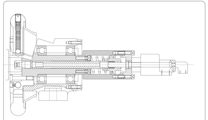
To provide continuous air pressure during the operation, the air shaft must be provided with a union which can remain engaged to the Safety Chuck side air supply during the entire operation. This application is useful in varying the air pressure to the air shaft during operation.
