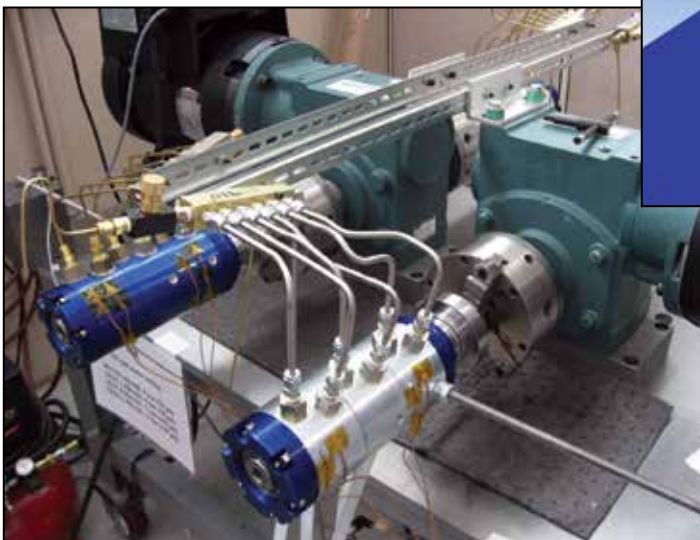
Deublin Multi-Passage unions testing fixture
